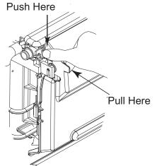
13 Remove water distributors from ice machine. Inspect each distributor for restricted orifice holes. Be sure all holes are full open.
